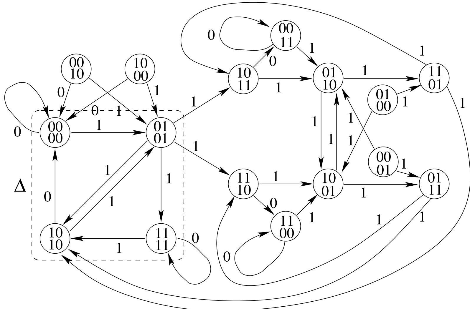
Any two-way infinite **path  $p$  in the pair graph** corresponds to a pair of paths in the original de Bruijn automaton with identical labels. These represent a **pair of configurations with the same image** under the CA.
