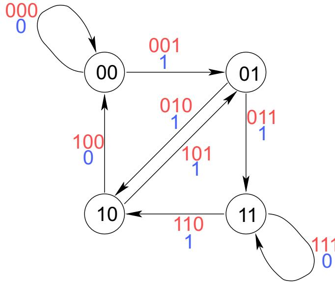
Infinite paths  $p$  in the de Bruijn representations provide **two** configurations:
