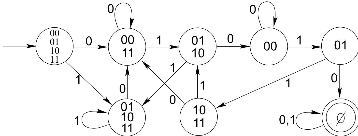
The shortest orphan is **01010**, given by the shortest path from the initial state to the final state.
