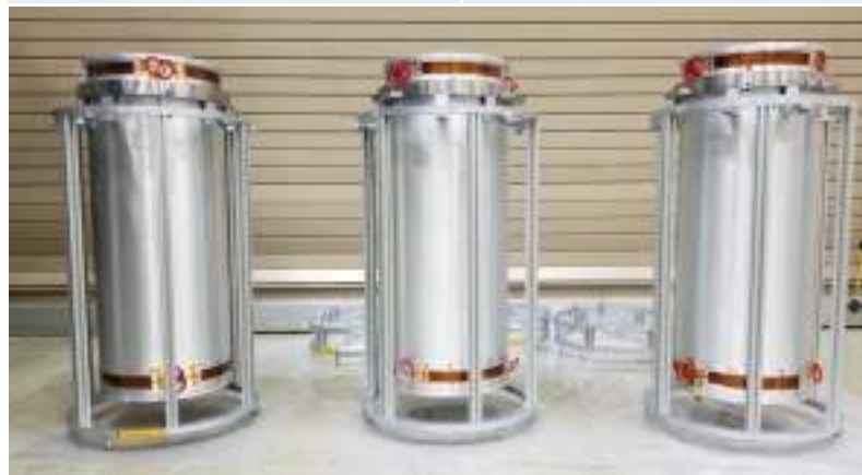
Three IXPE Mirror Module Assemblies
